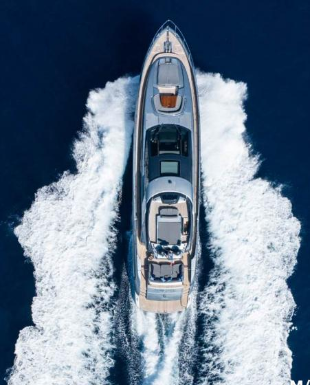
She is built with a GRP hull and GRP superstructure. With a cruising speed of 30 knots, a maximum speed of 38 knots and a range of 230nm from 7,500litre fuel tanks, she is a great combination of highperformance and style.
